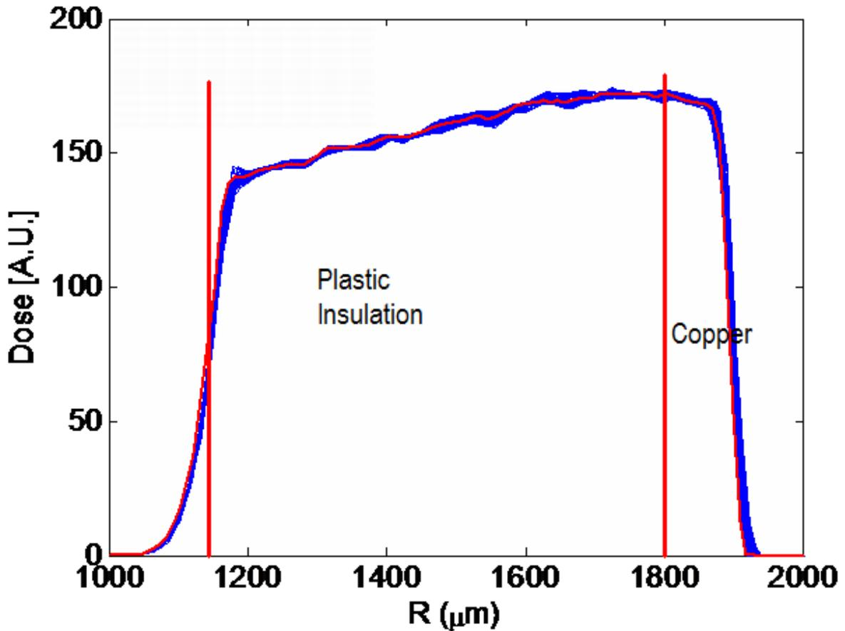
Figure 3. Monte Carlo simulations of dose as a function of radius for the case where the wire twists at least 30 degrees in the handling fixture. With azimuthal asymmetries removed, the best uniformity is achieved at 600 to 620 kV for 0.76 mm (0.03 inch) of insulation.
