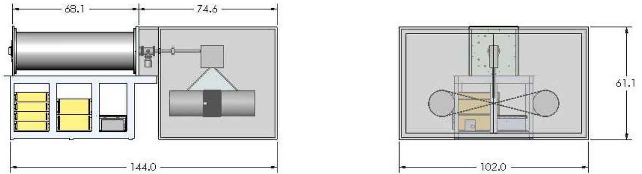
Figure 1a. Accelerator side view (left) and front view (right). The left view shows the cylindrical accelerator with control and power electronics underneath. The right view is a face view of the accelerator and side view of the capstan assembly.
