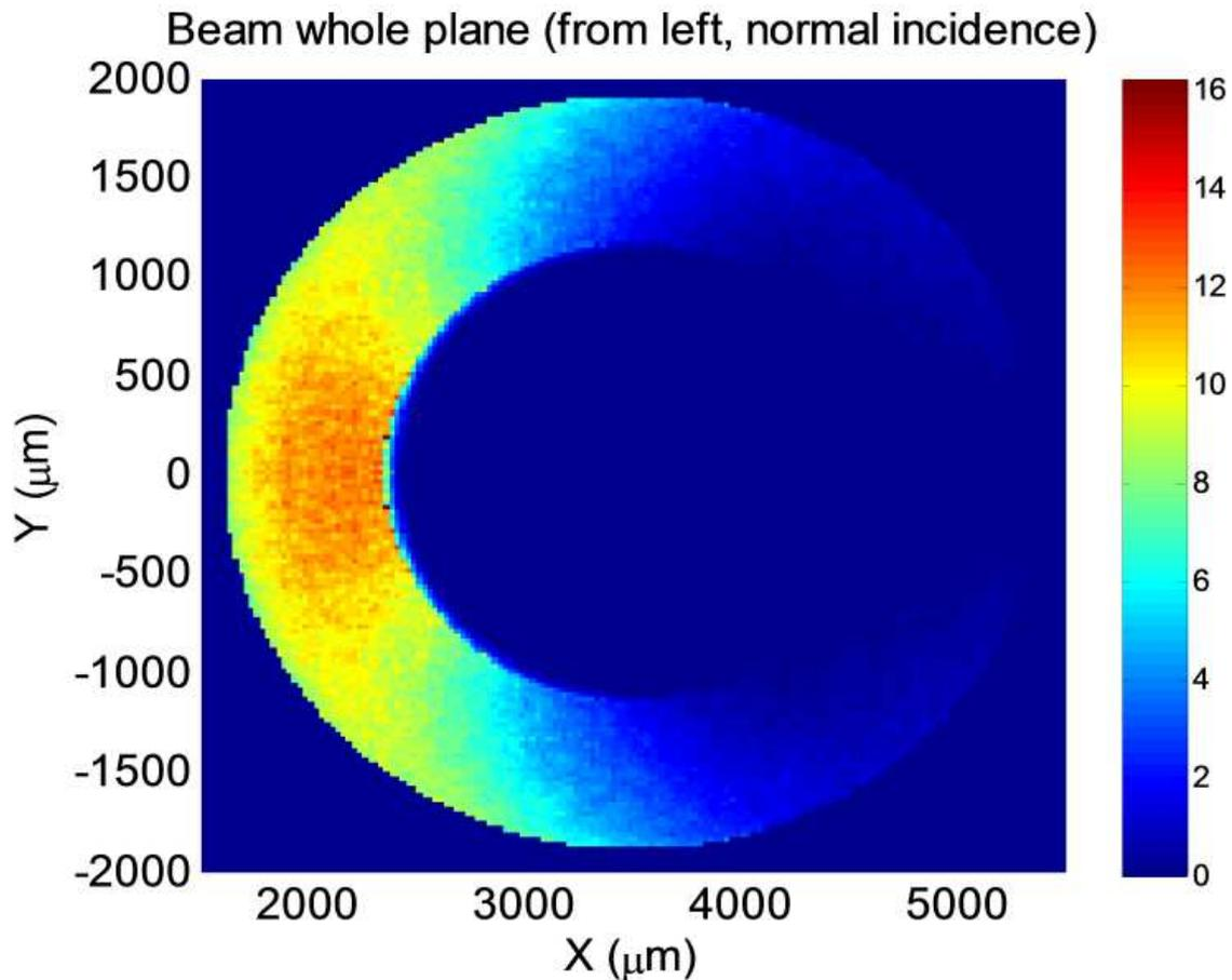
Figure 2a. Monte Carlo simulation of a planar electron beam impinging on flame retardant plastic coated #10 copper wire. The central circle is the copper. The region between the two circles is the plastic.
