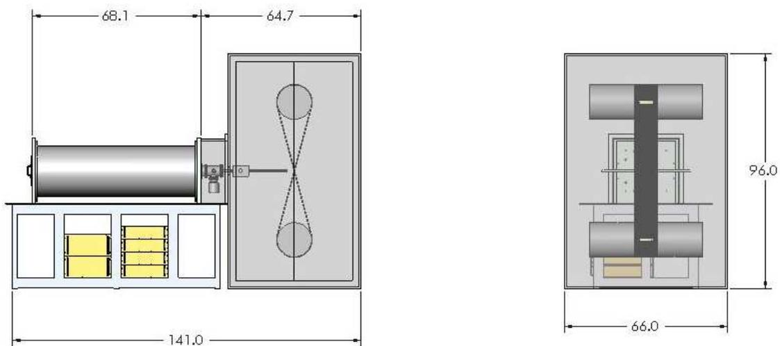
Figure 1b. An alternate variant on the size and positioning of the wire and capstan assembly.
