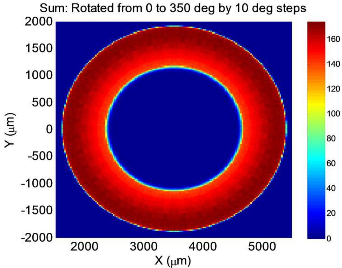
Figure 2b. Irradiated dose contours without twist from two sides at the figure-eight capstan cross-over point.
